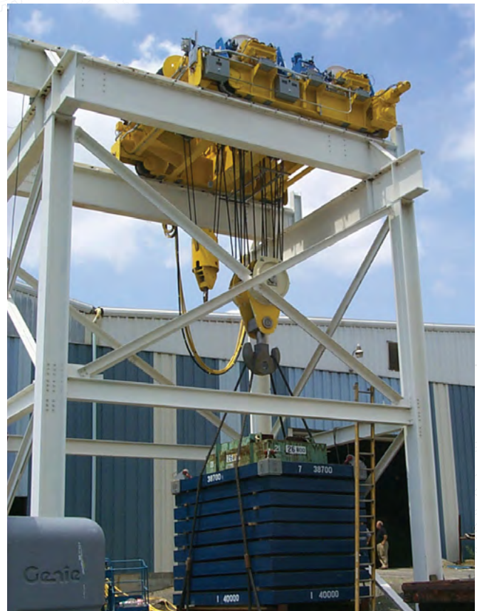
LOAD TESTED IN AMERICAN CRANE'S TEST TOWER
