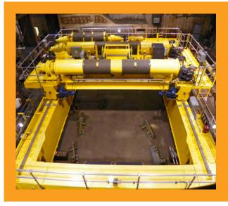
Multiple Girder Cranes are similar to single girder cranes but with multiple girders, typically two. Multiple girder cranes have several advantages over single girder designs. With the multiple girders, they can accommodate higher capacities and there is a hook clearance advantage, typically around 18-36 inches.
