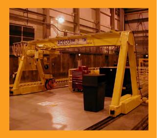
runway would require cannot be sacrificed, or in structures that cannot be economically modified to accommodate an overhead runway. In smaller applications, the runway may even be substituted with wheels, making it a very flexible option for smaller low use low capacity scenarios.
