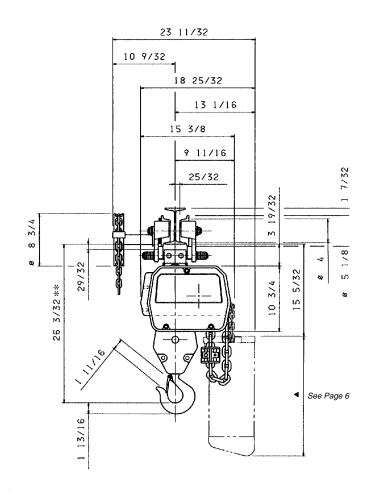
\*\* This dimension allows for 1" clearance between load block and underside of hoist.
