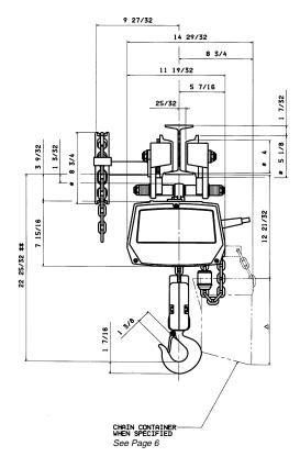
EC-3 (Geared Trolley) ECGT-2032 (1 Ton), ECGT-4016, ECGT-4024 (2 Ton) (Parallel Mount)
