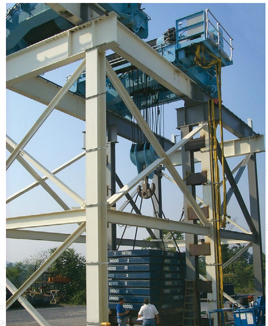
LOAD TESTING A TROLLEY IN OUR TEST TOWER
